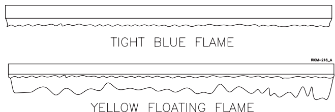
Figure 20 - Main Burner Flame
